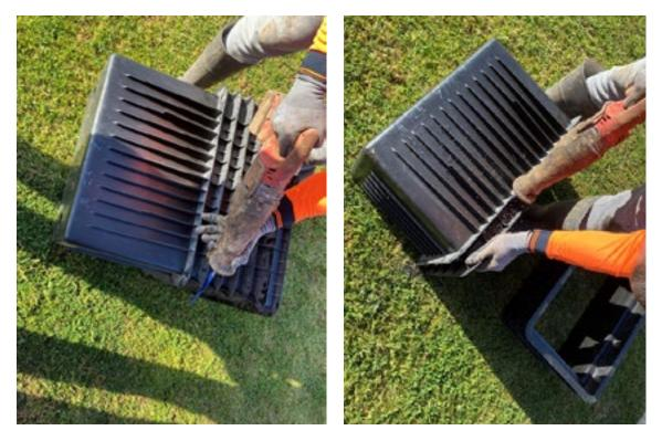
Important Step: The base half must be above the primary large rib. This Insures screws have a large area to grip.
